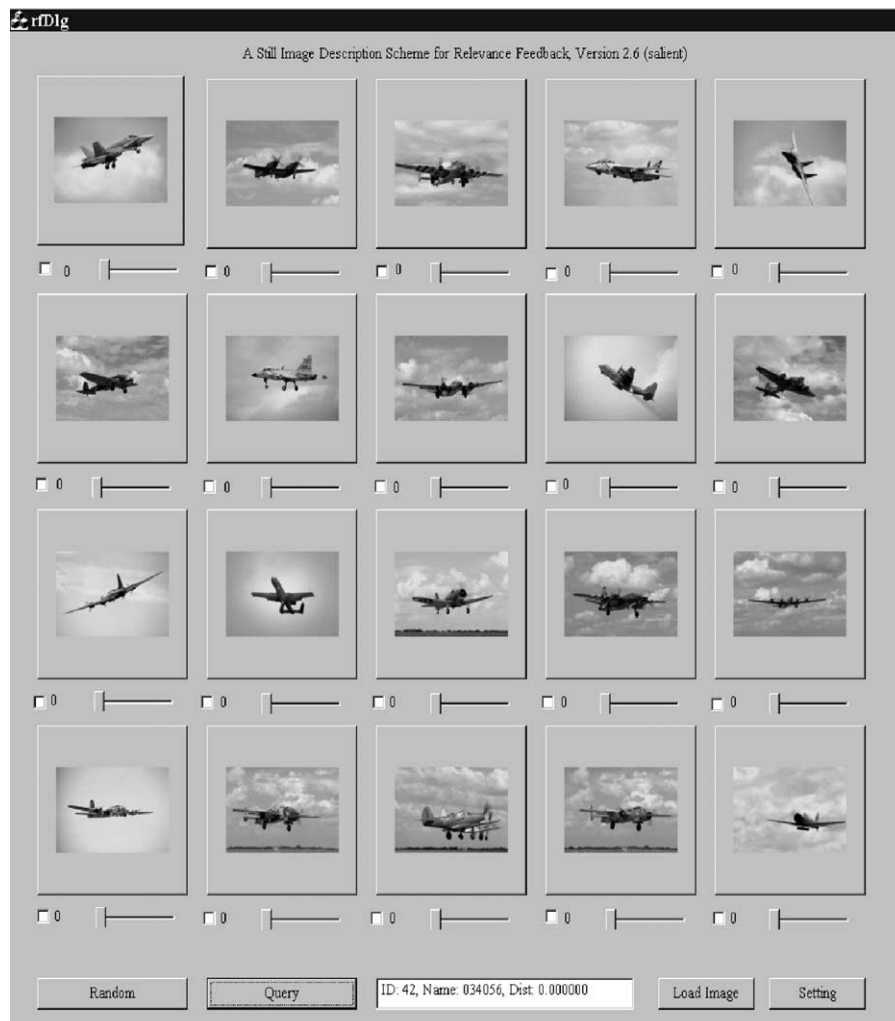
Fig. 4. An experimental result using the color moments extracted from the 3 \times 3 neighborhood of the Daubechies4 salient points (rank from the left to right and from top to bottom, the top left is the query image).
