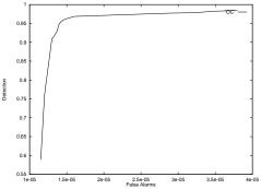
Figure 5. The operating characteristic for the face detector.
