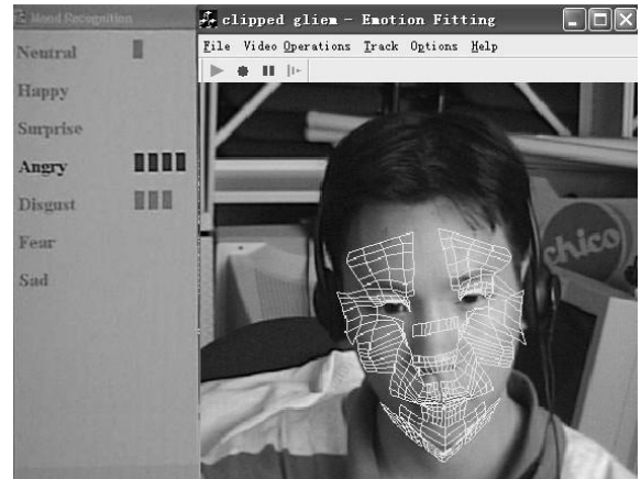
Figure 1: A snap shot of our facial expression recognition system. On the right side is a wireframe model overlaid on a face being tracked. On the left side the correct expression, Angry, is detected (the bars show the relative probability of Angry compared to the other expressions).
